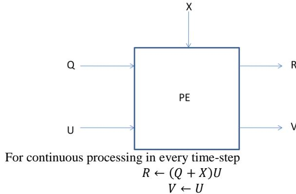
**Fig.4.** Function of each PE, except (N+1)th PE, of the systolic architecture-2 shown in Fig.3.
