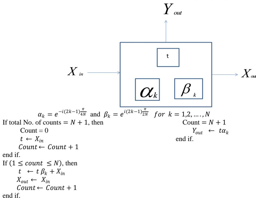
Fig.2. Function of  $k^{\text{th}}$  PE of the systolic architecture shown in Fig.1.
