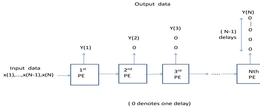
Fig.1. Systolic linear array architecture-1 for computing N-point DST-IV.
